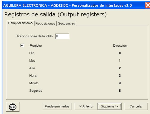
Any address can be customized, but the absolute address “0” should be assigned to allow the compatibility with installations with equipments with firmware series 1.
