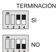
The connexion should be carried out in a "Daisy chain" configuration and only the end of line resistors of the equipments placed at the ends have to be enabled, whenever the impedance of the cable used is the same value as the end of line resistor.
